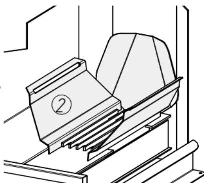
1) Install the back plate with a convex part to the wall of the firebox. The upper part of the plate shall rest on the firebox wall, while the lower part shall be spaced 5-10 mm from it;
