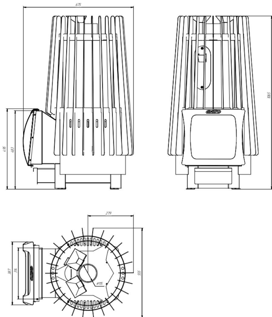
**Fig. 1** Dimensions of heater
