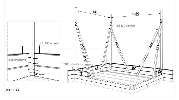
2.5 Continue to install the wall logs on top of each other according to the "Wall Layout" scheme on page 7. Use 6x180 screws to connect all wall logs to each other and 4.5x70 screws to fix all logs to corner posts, like shown in Scheme 2.3.
