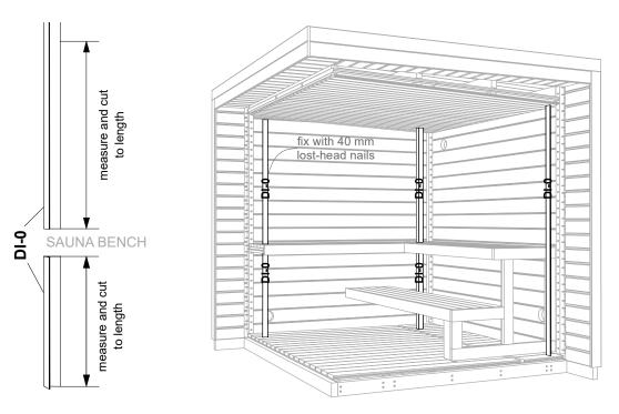
9.2 Measure and cut to length all DI-00 ceiling and floor moldings and fix them in place with 40 mm lost-head nails (Scheme 9.3).
