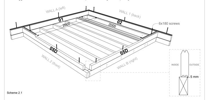
2.2 Place the second row of wall logs on top of the first row. Use a hitting block and a rubber mallet to set the logs in place. Attach the second row to the first using 6x180 screws and a battery drill. Suggestion: Pre-drill the holes for the screws to prevent wall logs from splitting.
