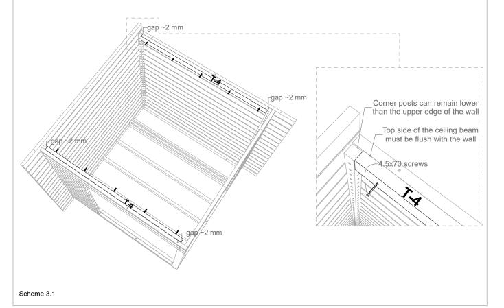
3.2 Temporarily lay one KL-1 roof board or some other straight detail on top of the front and back walls. Mark the diagonal that forms under the detail on the side walls with a pencil. These markings will determine the installation height of the T-3 ceiling beams. Measure out the distance from T-4 beams and mark the locations on both side walls, like shown in Scheme 3.2. These markings will indicate the spacing between the ceiling beams.
