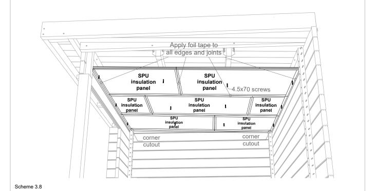
3.8 Place the DI-2 and DI-3 ceiling distance boards on top of the insulation panels and fasten them to the ceiling beams using 4.5x70 screws.
