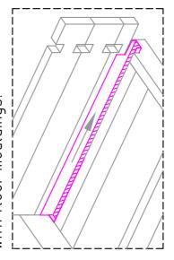
Fasten floor boards with screws from the tongue side of the board. First board should be placed "5mm from wall and when cutting last board make sure there is 5mm gap as well. Leave "2mm gap between floor board (cross cut sides) and walls. Lastly fix mouldings in place.
