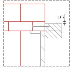
Framing should be 5mm inside from outer wall.
