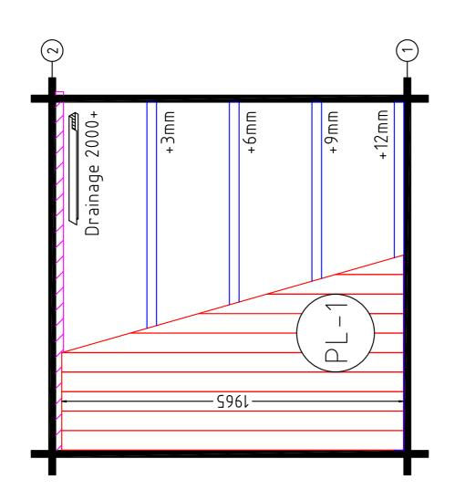
Fasten floor boards with screws from the tongue side of the board. First board should be placed ~5mm from wall and when cutting last board make sure there is 5mm gap as well. Leave ~2mm gap between floor board (cross cut sides) and walls. Lastly fix mouldings in place.
