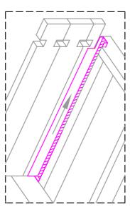
When placing drainage, fix closed end temporarily ~5mm higher than opened end to guarantee slope towards outer wall for water. After placing floor boards fix it permanently with floor mouldings.
