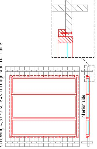
4. Fasten mouldings with 3x40 screws. Mouldings on sides should cover about 10mm and upper moulding should cover about 20mm.
