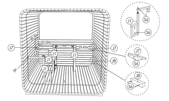
**STEP13:**Install sauna benches on top of legs (J; J3; J4; J5). Bench cross boards have to match the tops of the bench legs. Check distances from walls, then fix benches on the legs.
