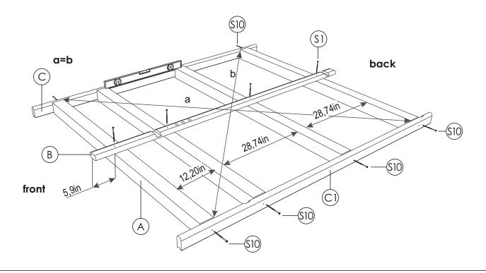
**STEP 2:** Drill 0,39in hole in each plank,in the front wall groove and in the rear wall groove to the out-side. Fix 2 board panels (C2; C3) with 5x100 ss screws (S1) to each side from the centre stave. Use 8 screws for each panel as shown in picture. Between panel and stave use foam for better insulation.
