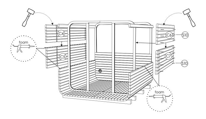
**STEP 10:** Fix the next body staves (C; C1) and board panels (C2;C3) on both sides with foam between the stave and panel with screws 4x60(S10) for each side. Use a rubber hammer if necessary, possibly need to push a bit back and front panels.
