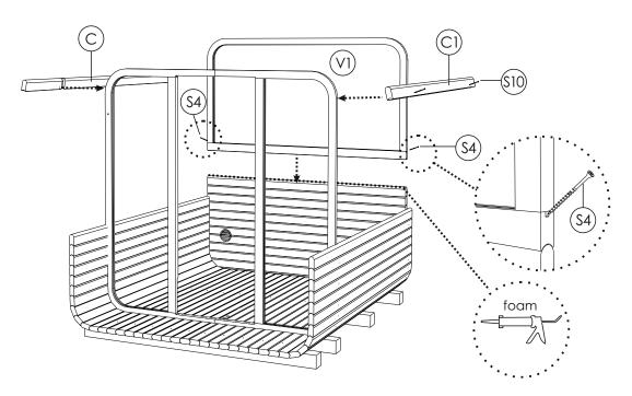
**STEP 9:** Fix the next board panels (C4; C5; C6; C7) on both sides with foam between the stave and panel with screws 4x60(S10) for each side. Use a rubber hammer if necessary, possibly need to push a bit back and front panels.
