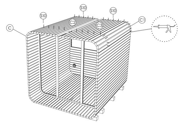
STEP11: If needed, use thinner staves (H1) to fill the gap between (H) staves and apply foam between staves. Install metal bands over the screw holes, then tighten the band.
