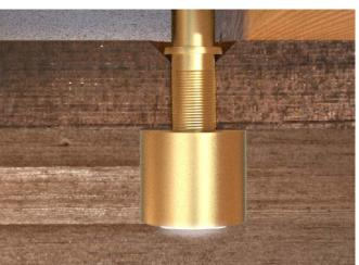
The heater lens is typically installed into the ceiling on top of the stove to illuminate the steam and the heater. The diameter of the light cone changes when the lens is screwed towards the end of the fiber. The deeper you rotate the lens, the wider the cone becomes. It's good to take this into account when counter-drilling.
